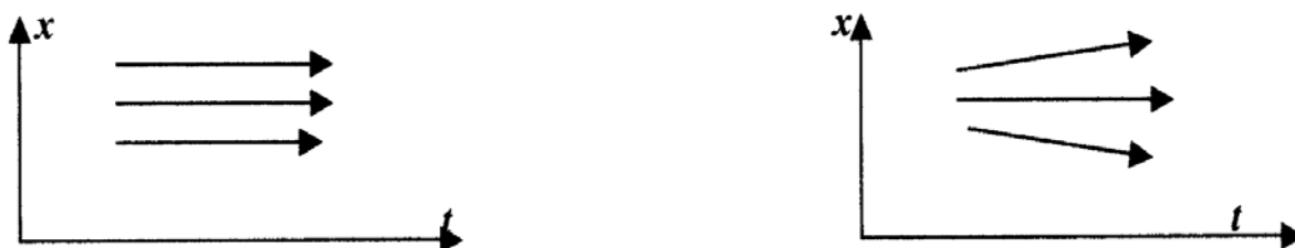
Figure 4. If the space properties are not changing in the time, a closed system energy is constant (at the left). If the space properties are changing in the time, a closed system energy is not constant (at the right)
